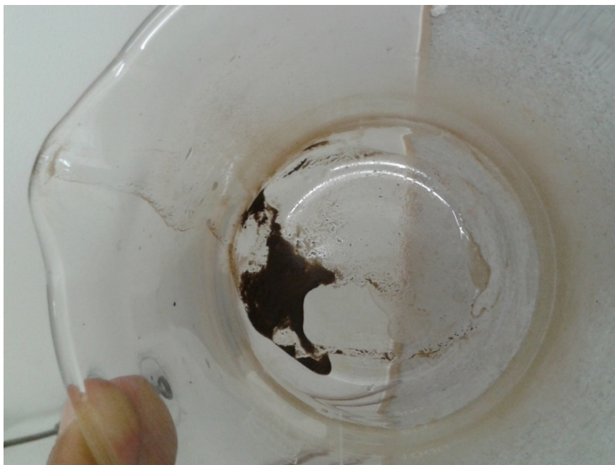
Figure 2.36. Particles extracted from the heating coil
