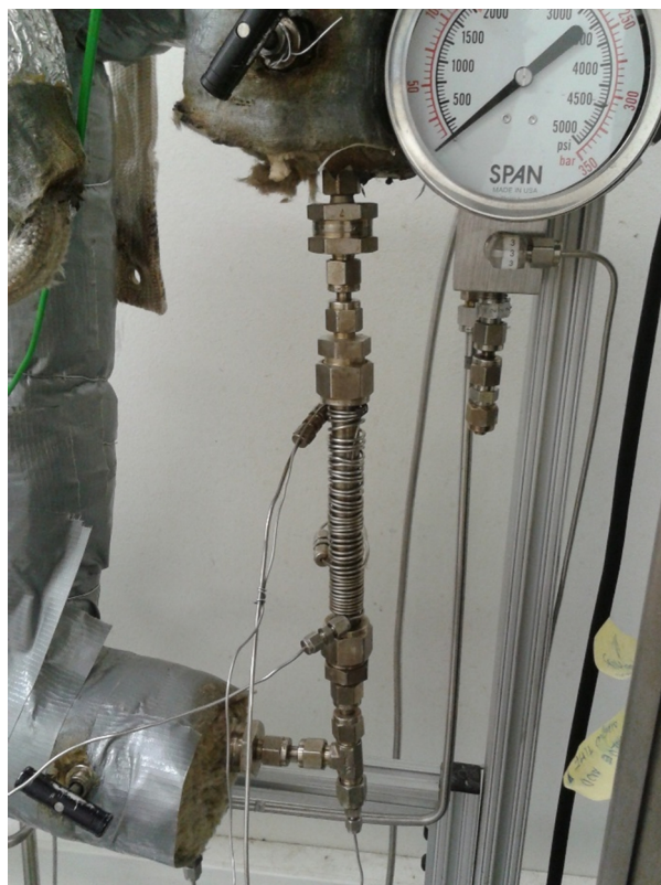
Figure 2.39. Dissolution Reactor and its cooling line in detail.
