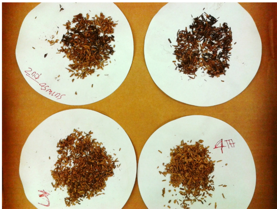
Figure 3.2. Recovered Spruce for the four different reaction times at 225 DegC. Top Right: 60 min. Top Left: 45 min. Bottom Left: 30 min. Bottom right: 15 min.
