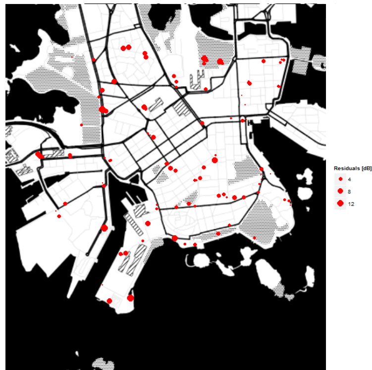
Figure 49: Bubble plot of the residuals, after they have been back transformed to the original units, as usual, these are bigger where less samples have been taken.
