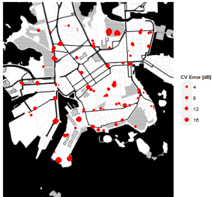
Figure 39: 1-fold crossvalidation using Simple Kriging. The bubbles indicate the difference in absolute value between the local prediction in a sampling location if the dataset had not contained that measurement. It is possible to visualize that most of the errors are concentrated on the borders of the sampling area, where fewer samples are available.
