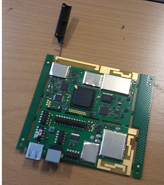
Figure 6: Detector board equipped with the UHF antenna.
