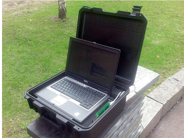
Figure 4: Measurement setup in the Helsinki campaigns, consisting of a waterproof case containing a portable computer connected to the detector via USB.
