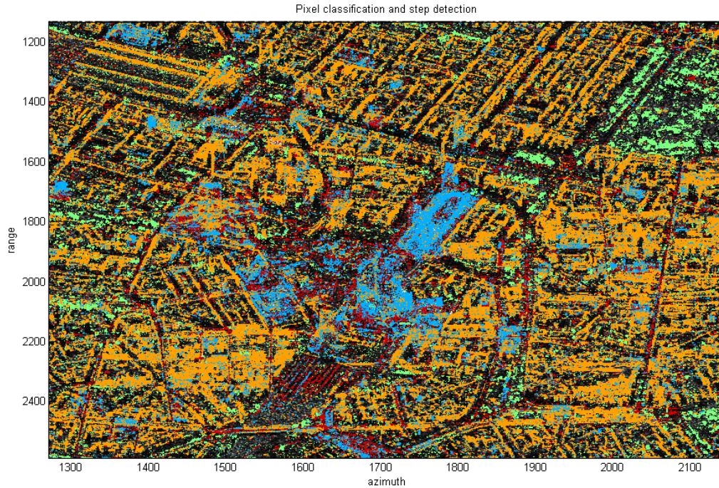
Figure 4.15: Pixel classification and step detection on piazza Gae Aulenti and the Porta Nuova area. In blue are the pixels characterized by step detection. In green are vegetation pixels, in orange building pixels and in red road and square pixels.
