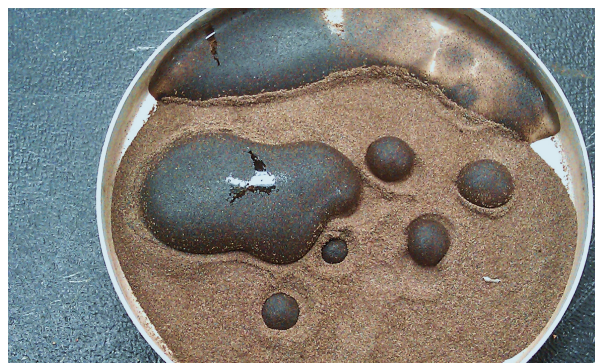
Figure 4.3: The fine material (with grains smaller than 75 \mu\text{m} ) presents a hydrophobic behavior when dry. The picture shows some droplets of water on the surface of the fines.
