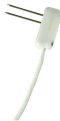
Figure 3.4: Two-needle probe SH-1 of the thermal properties analyzer KD2 Pro by Decagon (reproduced from [67]).
