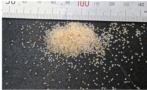
Figure B - I: Sample of coarse silica sand, Accusand C-190 (by Unimin Corp.), d_{50} = 0.73 \text{ mm} , \rho_s = 2.66 \text{ g/cm}^3 .
