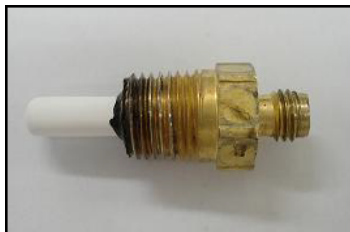
Figure 3.2: Tensiometer with porous ceramic cap. Reproduced from [32].
