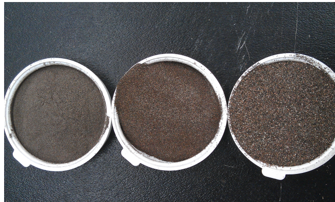
Figure 4.2: Fine components of fresh green roof soil. The jar in the left contains the particles smaller than 75 \mu\text{m} . The jar in the middle contains the particles retained by the 75- \mu\text{m} mesh. The jar in the right contains the particles retained by the 106- \mu\text{m} mesh.
