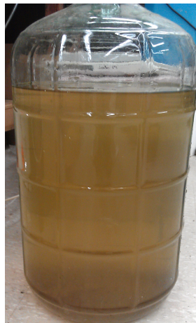
Figure 4.6: Water collected in the tank after that the column was flushed with 19 liters. Deposition of fines can be observed at the bottom of the tank.
