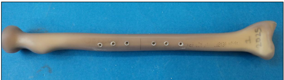
Figure 84: Sample belonging to the HybSYK3.5mm group ready for testing
