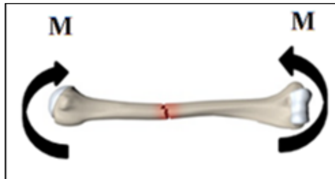
Figure 41: Transverse fracture on a long bone produced by a bending moment [67]
