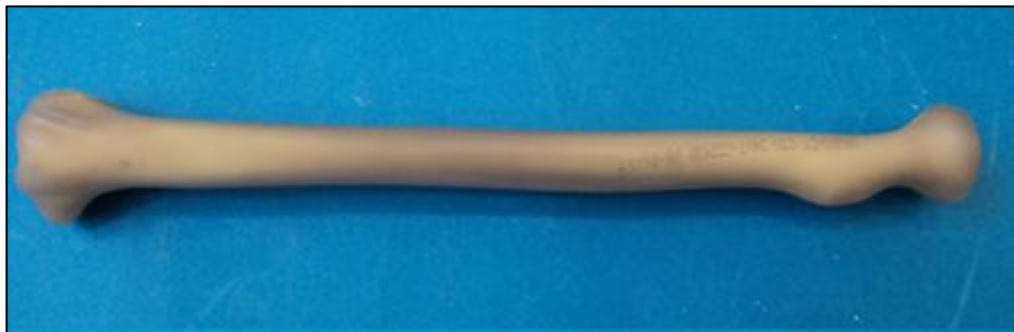
Figure 82: 4 th generation composite radius bones
