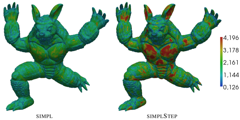
Figure 5.14: Simplified mesh up to 40% of the initial number of vertices, on the left the one obtained with SIMPL, on the right the one obtained with SIMPLSTEP, for each node v_i we provide the maximum length of the edges connected to v_i .
