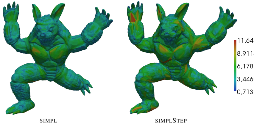
Figure 5.16: Simplified mesh up to 5% of the initial number of vertices, on the left the one obtained with SIMPL, on the right the one obtained with SIMPLSTEP, for each node \mathbf{v}_i we provide the maximum length of the edges connected to \mathbf{v}_i .
