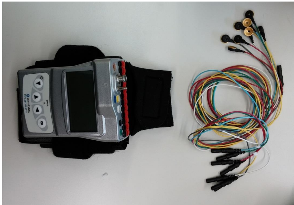
Figure 3.1: EMBLA titanium™ device allows to get signals (EOG, EMG, ECG, EEG) from 9 different channels.
