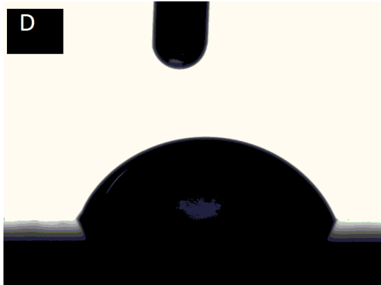
Fig 5.3.D contact angle on 275.D.Na
