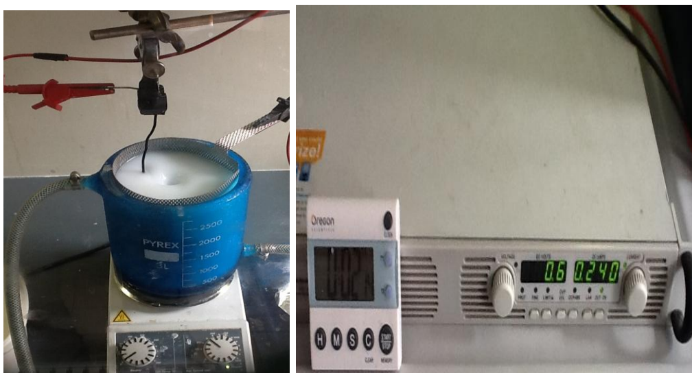
Fig 4.3 ASD experimental set-up (Left), DC power supply (Right)
