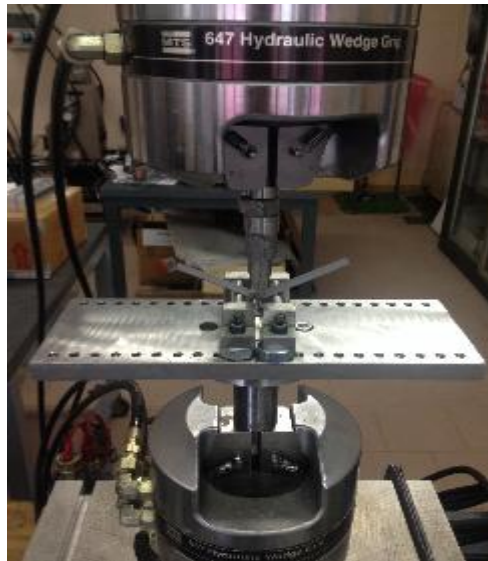
Fig 5.4.17 sample during 3 point bending test
