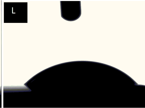
Fig 5.3.L contact angle on 185.D.Na
