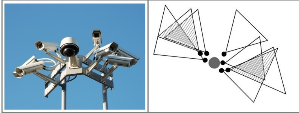
Figure 4.1: Public area, camera nodes, overlapped field of view
