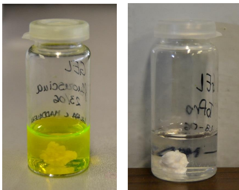
Figure 3. 38: Hydrogel loaded with Fluorescein (a) or To-Pro3 (b) immersed in 4 mL of PBS.
