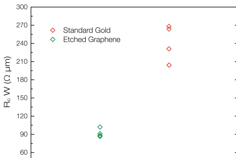
Figure 4.11: Contact resistance measured in case of standard gold electrodes compared to etched contacts.
