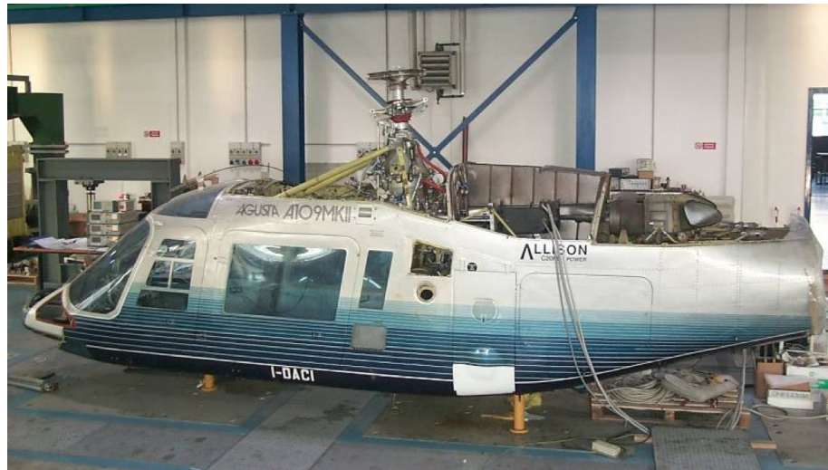
Figure 1.6: Helicopter fuselage employed during the Friendcopter project.
