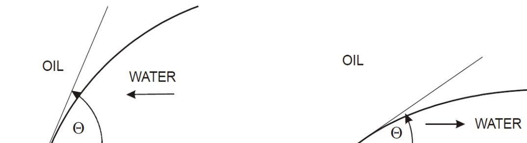
Figure 1-11: contact angle in a water wet reservoir. Left: wetting phase is increasing (imbibition). Right: wetting phase is decreasing (drainage). L. P. Dake; *Fundamentals of Reservoir Engineering*.
