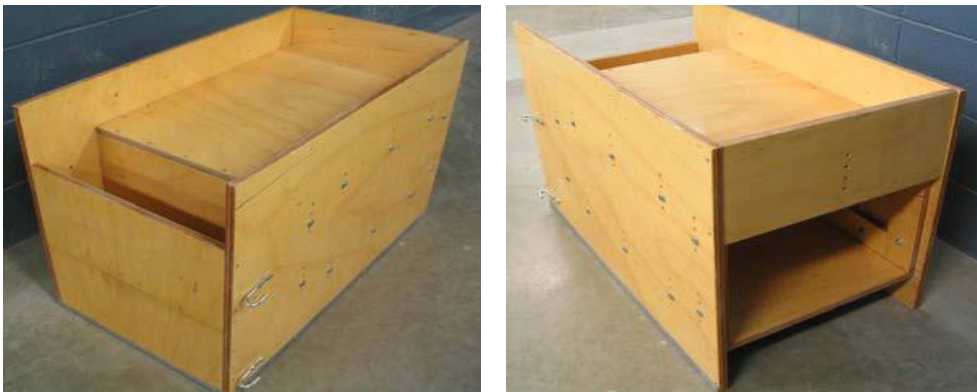
Figura 2.24 Mini slip-form per lo studio del Self-Compacting Concrete – Application for slip-form paving
