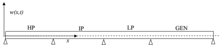
Fig. 34 – Shaft of a steam turbine + generator scheme
