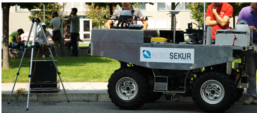
Figure 2.5: The robot, before the work of this thesis, with the drone parked on its platform. On the left it is possible to see the ground station for the RTK correction
