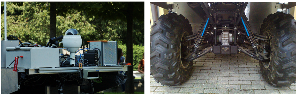
Figure 2.7: Two of the sensors that are still installed on the robot but not currently used: the omnidirectional camera (left) and the linear potentiometers (right)
