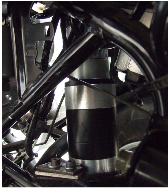
(a) The Intecno ND180.240 motor that controls the steer
