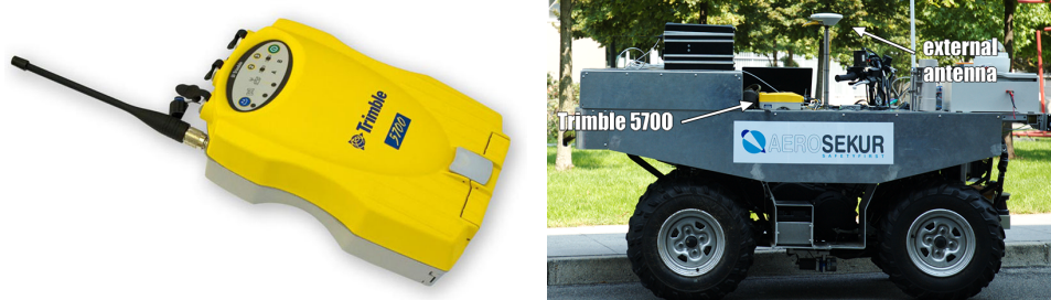
Figure 3.3: The Trimble 5700 (left) and its position on the robot with the external antenna (right)
