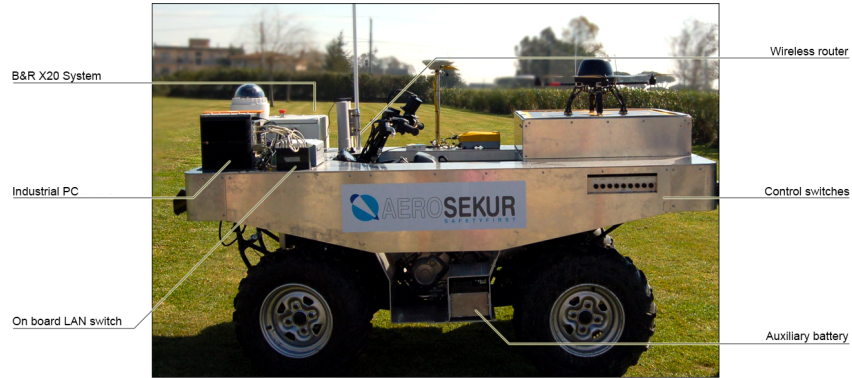
Figure 2.6: The position on the robot of its main components
