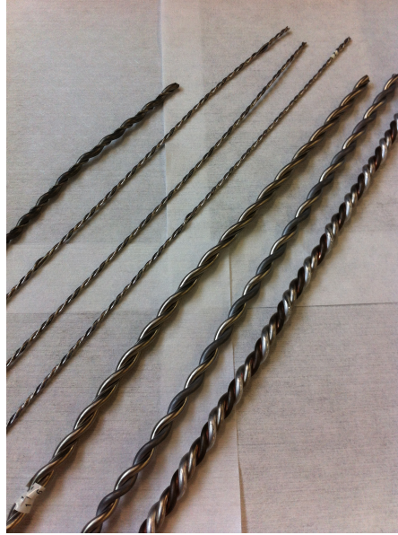
FIGURE 3.7: Examples of some of the cathodes used for the realization of the NEG thin film coatings tested.
