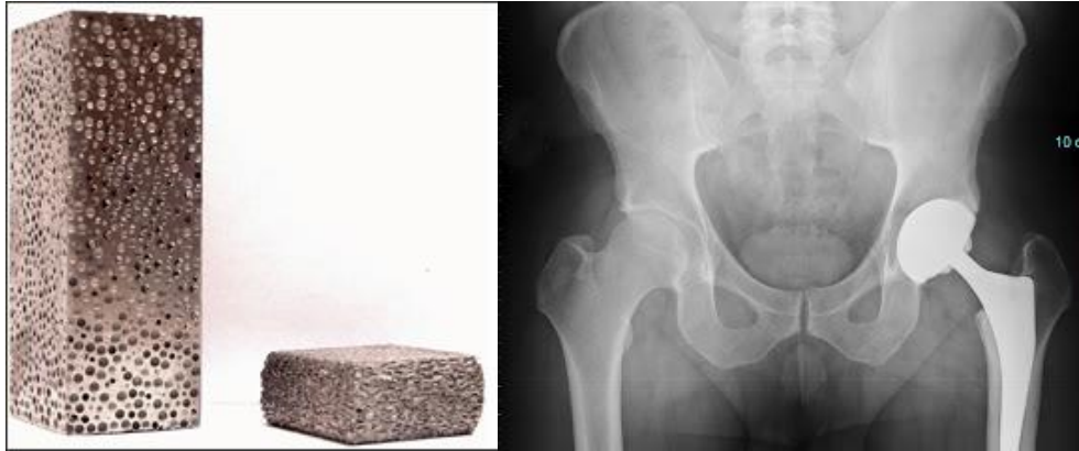
Figure 1.22: Titanium made by preformed hollow spheres used for a hip prosthesis. [13]
