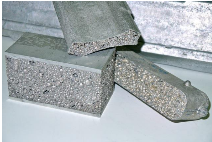
Figure 1.20: Aluminum foam components for crash absorption in automotive industry [11]
