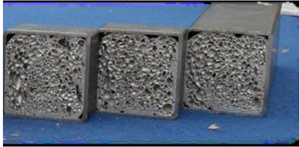
Figure A 1: Sections of foam filled steel tubes and partial detachment of the foam
