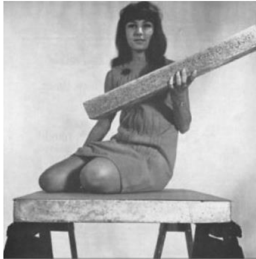
Figure 1.17: Bjorksten demonstration of both lightness and stiffness of Al foam [1]
