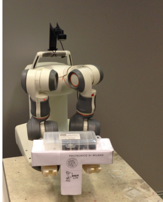
Figure 6.7: The ABB FRIDA dual arm robot prototype lifting a tray with an object laying on it.
