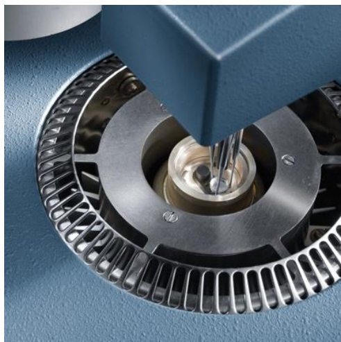
Figure 23. In DSC Q2000 already analyzed samples are removed and replaced automatically. Close to that a sapphire sample is housed. According to temperature transitions, heat flow variations with respect to the reference material occur to keep both materials at the same temperature.
