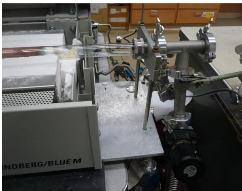
Figure 42: (b) Particular on the right side of the deposition chamber showing the valve (in black) connected to the vacuum pump
