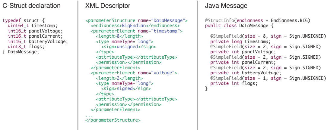
Figure 2.4: Physical to logical attribute mapping in the Classic PerLa Middleware. The annotations added to the Java Message allow the Marshaller and Unmarshaller components to encode and decode the information exchanged with the remote device.
