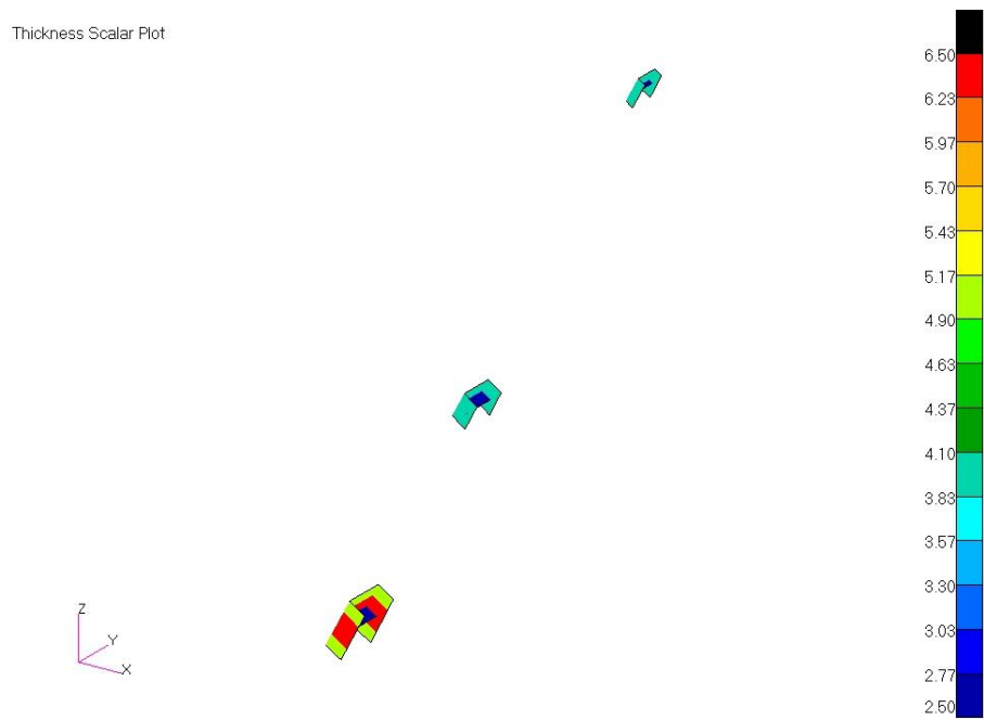
Figure 70: Hinges: thickness distribution
