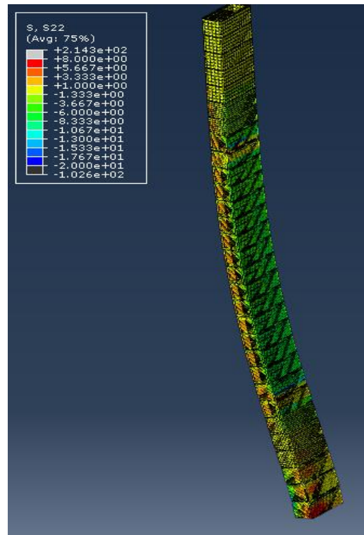
Figura 8-10- Axial stress at collapse - reinforced panel clamped at the basis
