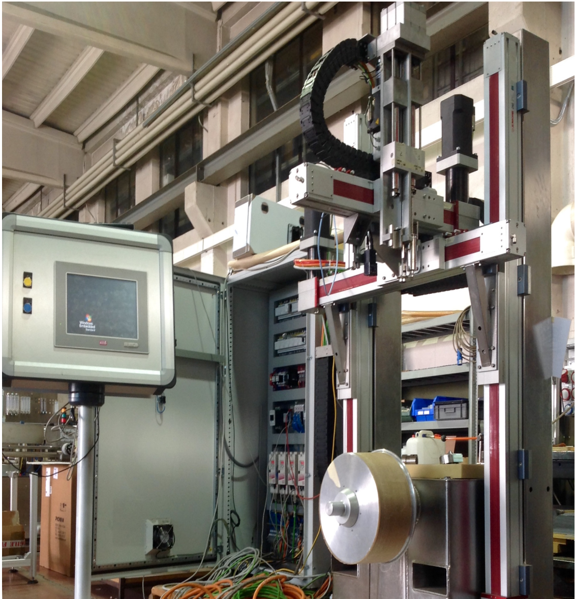
Figure 15. Dry-wet spinning apparatus
