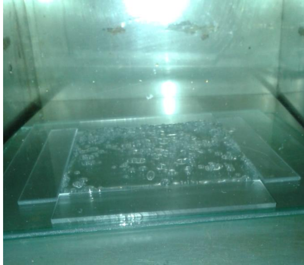
Fig. 2.12 Silicone rubber during degasification process
