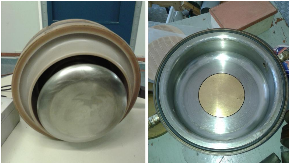
Fig. 3.10 The upper plate (left) and the lower plate (right) of the test cell capacitor
