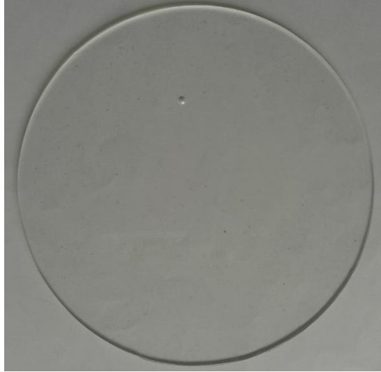
Fig. 3.16 The specimen D of Bluesil ESA 7250
