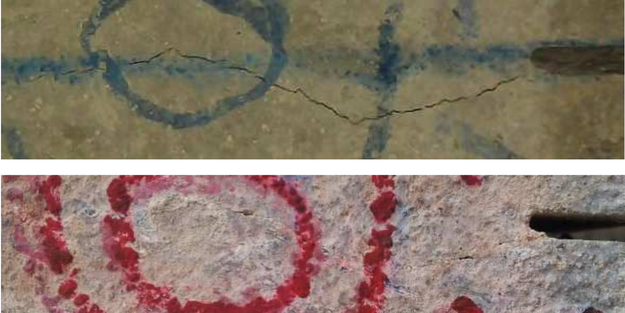
Figure 50: level of crack sealing after 90 days of conditioning for specimens precracked up to 600 \mu\text{m}
