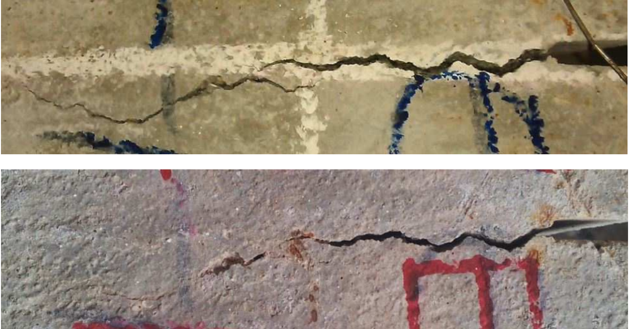
Figure 62: level of crack sealing after 90 days of conditioning for specimens precracked up to 4000 \mu\text{m}
