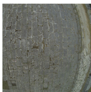
Foro 10 m GSD: 0.005 m Residui sui GCPs: 0.01 m Residui sui checkpoints: 0.01 m Differenza modello: +/- 0.02 m
