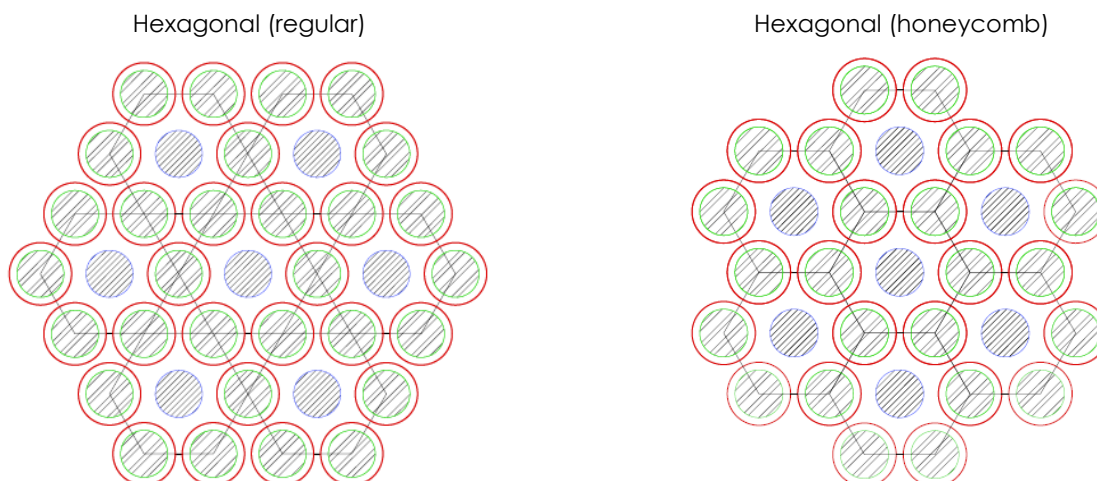
Figure 7.9 Modular configurations for reactor scale-up. Filling hatch is different for internally and externally irradiating UV lamps, loose in the former case and dense in the latter.
