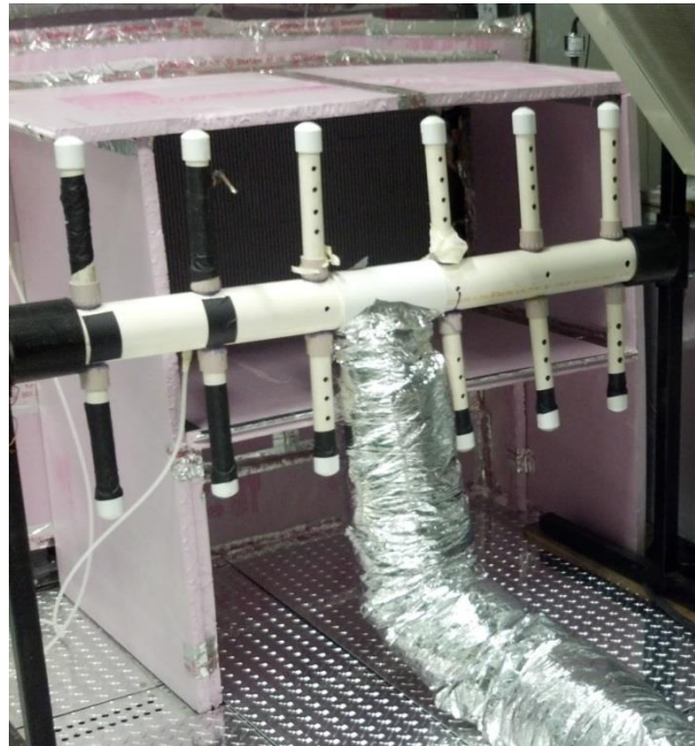
Figure 5.2 Picture of the air sampling device
