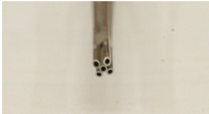
Figure 2.1 Close-up of the five hole pressure probe tip used for the experiment.
