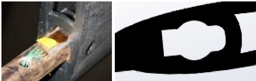
Figure 4.13 Detail of the design that allows not to damage the strain gauges while sliding the blade section onto the main spar.
