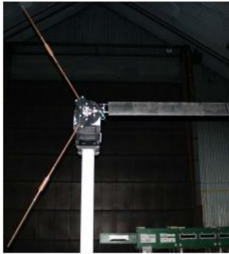
Figure 4.9 Frontal view of the assembled test rig with rotor installed
