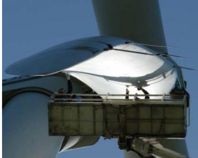
Figure 1.6 Multi hole pressure probe on 3.6MW size wind turbine (7).
