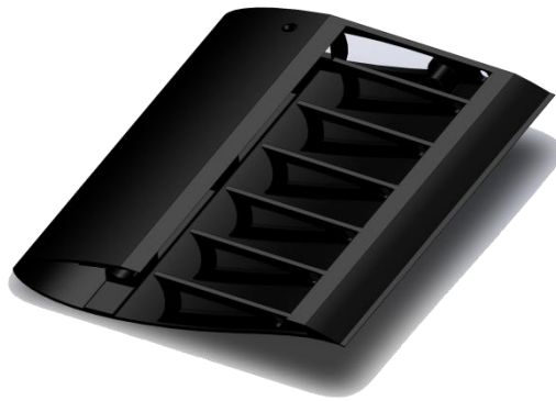
Figure 4.10 SolidWorks™ model showing the internal present design of the blade sections.
