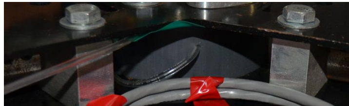
Figure 4.20 Reference pressure line into the hub spacer.
