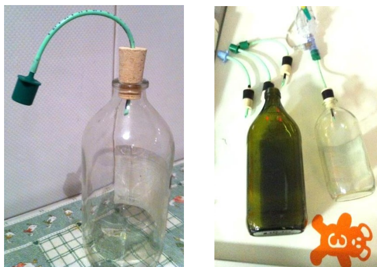
Figure 4.14 Test lungs setup to flow-dependent resistance compensation. A) Intubated test lung with a cork, B) different size bottle and ETT used for the in vitro study.
