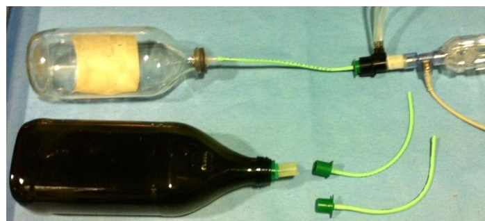
Figure 4.1 Different size bottle and ETT tube used for the in vitro study.
