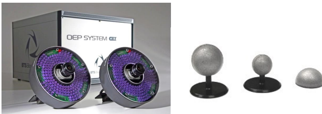
Figure 3.5 BTS Bioingeneer optoelectronic hardware, in particular a) 2 infrared cameras and the computer; b) reflective markers. In this study are used the hemispherical ones (the latter).
