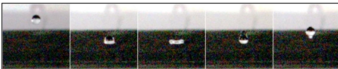
Fig. 68: Drop impacting on superhydrophobic surface of C12P_7 sample.
