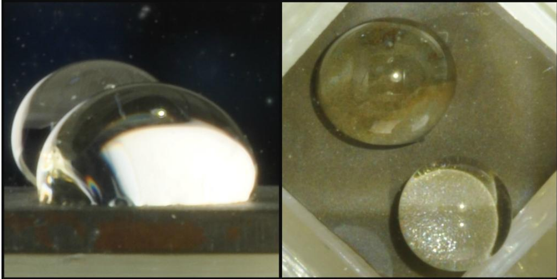
Fig. 55: Side and top views of two drops deposited on area with different deterioration grade.
