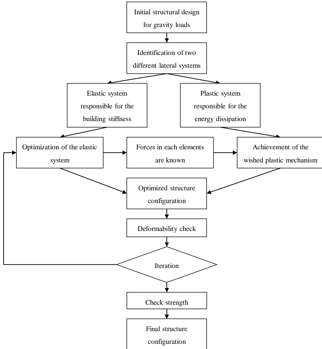
Figure 78: Workflow for the Tied Lateral System design
