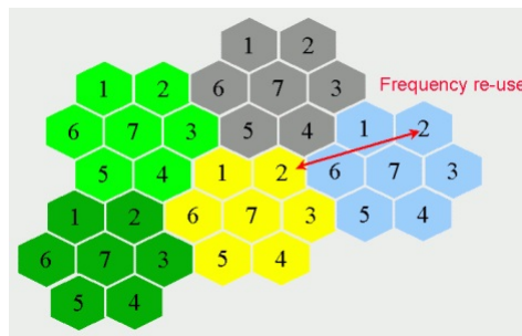
Figure 3.5: Frequency reuse in a cellular network (from www.telecomabc.com )
