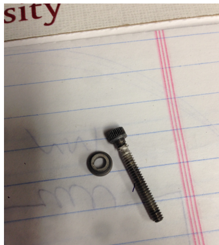
Figure 5.58: AFITr Cathode Keeper screw and shoulder insulator damaged.
