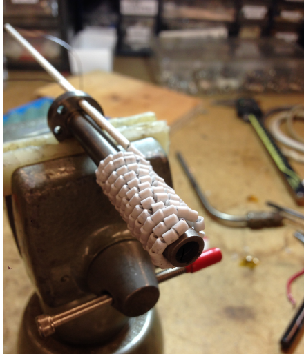
(a) Heating Filament assembling.
