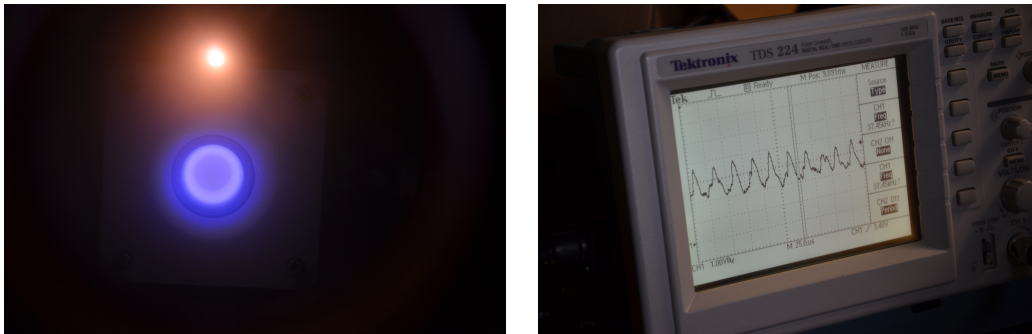
(a) CHTr running in glow mode w/o B field. (b) 40 kHz anode current oscillation.
