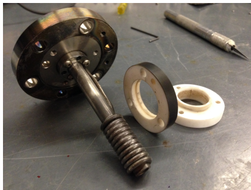
(a) Coated ceramic insulating elements, with original heating filament.
