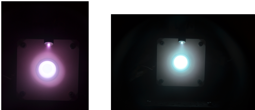
(a) CHTr running in glow mode w/o B field. (b) CHTr running with B field.
