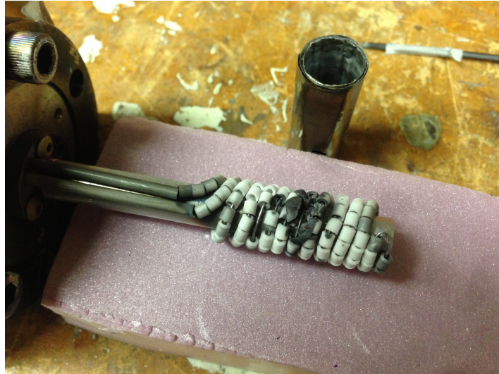
Figure 5.57: new AFITr Cathode heater damaged.
