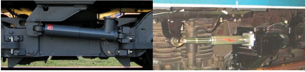
Figure 3.1: Anti-yaw damper, secondary yaw control: passive and active approaches
