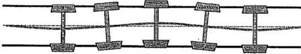
Figure 1.2: Hunting motion: the center of motion of the wheelset describes a sinusoidal path
