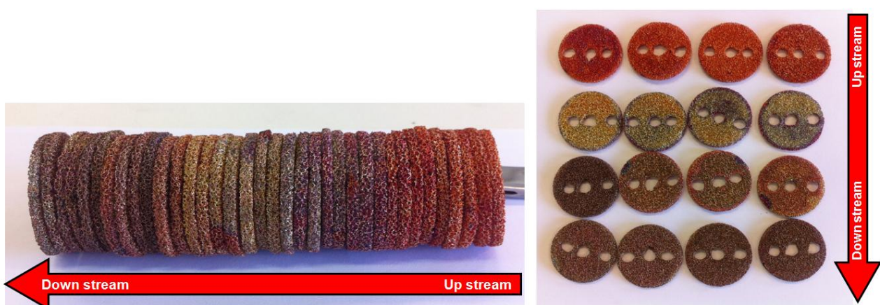
Figure 3.23 - Digital pictures of oxidized copper.
