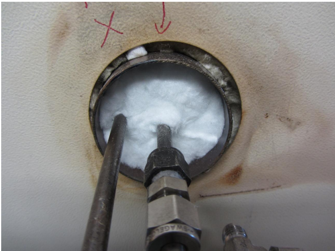
Figure 3.7 - Digital photograph of the insulation part, with the channel for the fourth thermocouple (pipe at the left) and gas inlet (central pipe).
