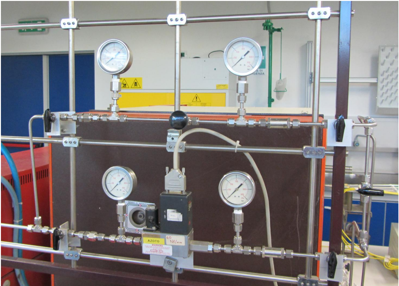
Figure 3.2 - Digital photograph of control section of the setup with a mass flow controller in parallel with a needle valve.
