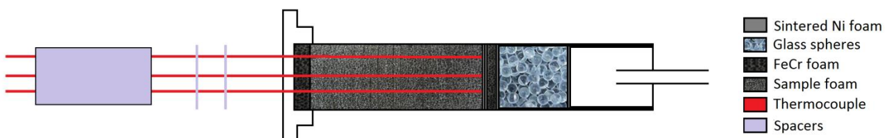
Figure 3.13 - Sketch of tube configuration with the two spacers.
