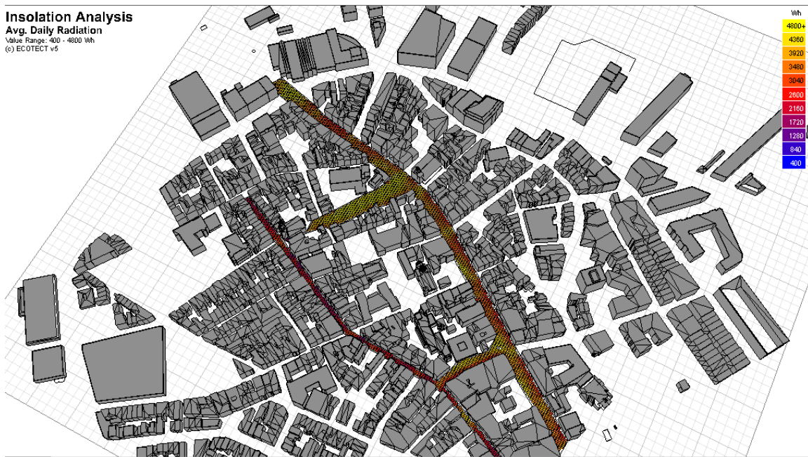
Figure 1-14: winter solar access analysis
