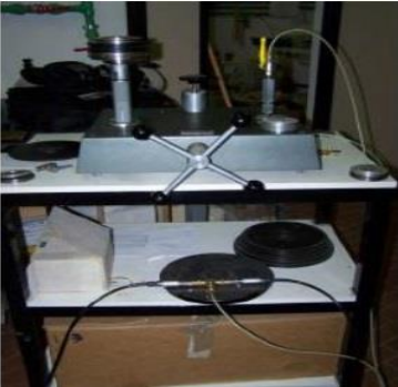
Figure 3-11: Pressure cells connected to the pump for generating hydraulic pressures.
