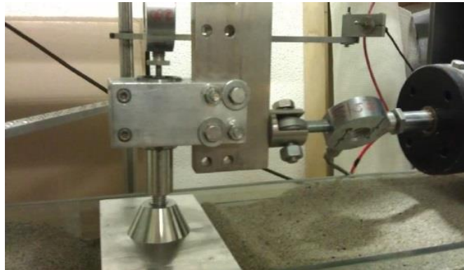
Figure 3-14: connection system of the shallow foundation.
