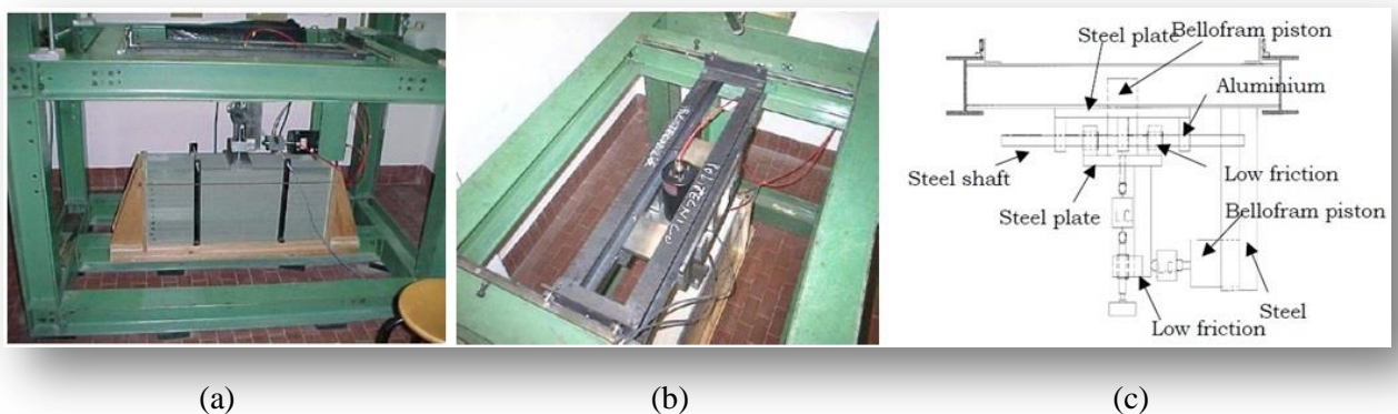
Figure 3-1: (a) front view of the loading steel frame and of the testing box, (b) upper view of the loading steel frame, (c) displacement transducers at the beginning of the tests.
