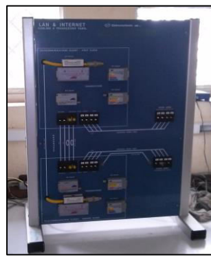
Fig. 4.13 Lan&Internet Connection Panel
