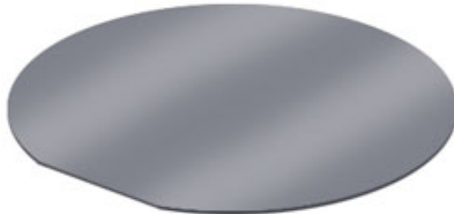
Figure 6 : Simple layout of a p-doped silicon wafer, with a 40 nm Pt coating
