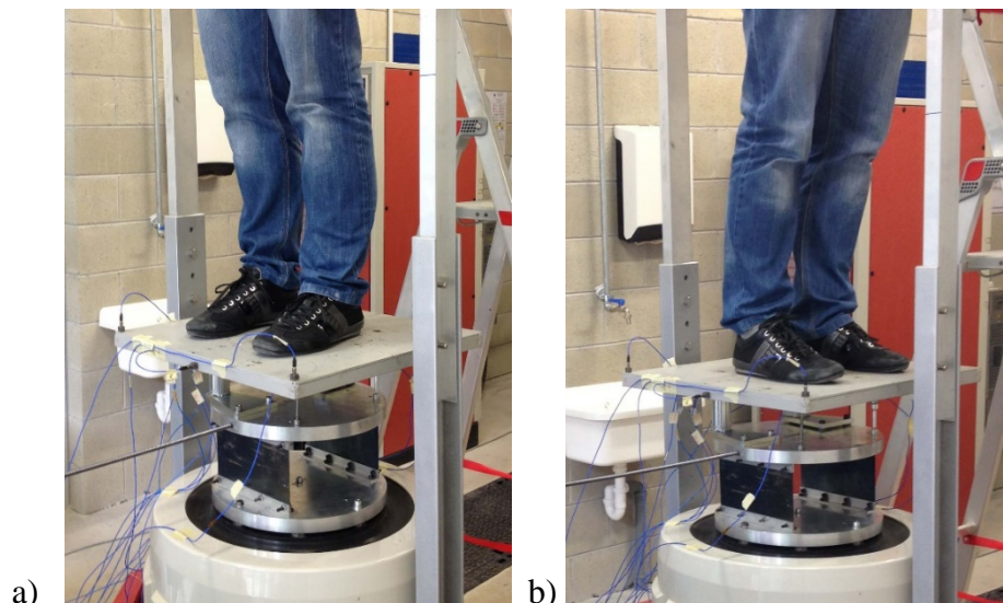
Figure 6.3 Position of the subjects on the force plate: a) frontal and vertical excitations, b) lateral excitation.
