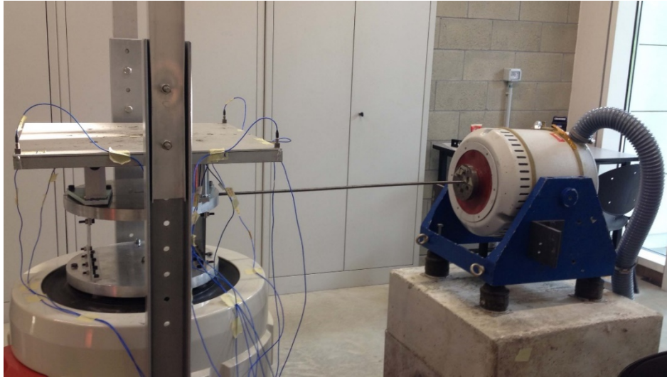
Figure 6.1 Experimental setup for the excitation and the measurement of the human body response in the basicentric reference system.
