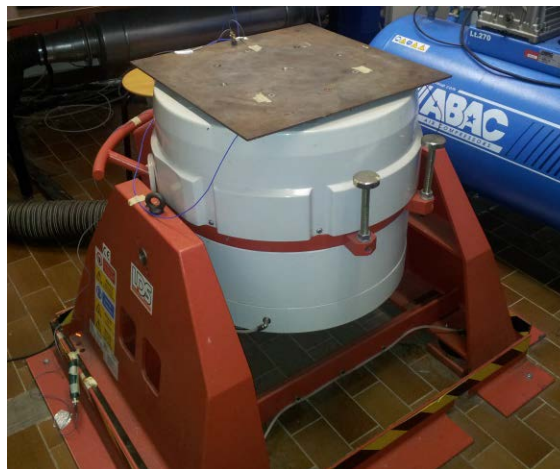
Figure 2.1 Snapshot of the laboratory instrumentation for the characterization of the apparent mass.
