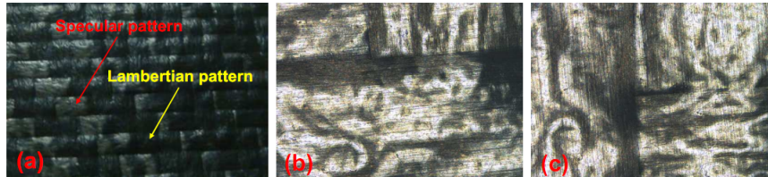
Figure 3.25: (a) Patterned Lambert+specular sample and acquisition result when rotation axis parallel to (b) x-direction and (c) y-direction.
