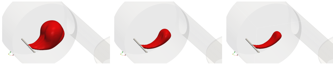
Figure 7.26: Average flame position ( G = 0 ) for the 1250 rpm, peripheral spark position case with different mixture compositions: images are shown with increasing air-fuel equivalence ratio (1.0, 1.3 and 1.5) from left to right at 355 CAD.
