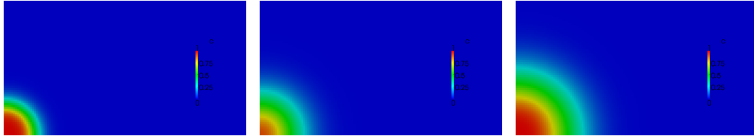
Figure 4.15: Sequence of images which portrays the evolution of the flame for FSD-CFM2-a model. The images show the progress variable profile for three time steps in succession (Time = 0.5 ms, 3.0 ms, 4.0 ms).
