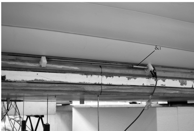
Figure 7.11: Full scale panel instrumentation: LVDT used to measure the superior longitudinal displacement of the upper TRC layer.
