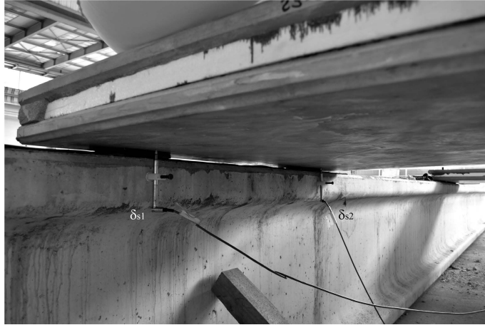
Figure 7.9: Full scale panel instrumentation: LVDTs used to measure the vertical displacement next to the supports.
