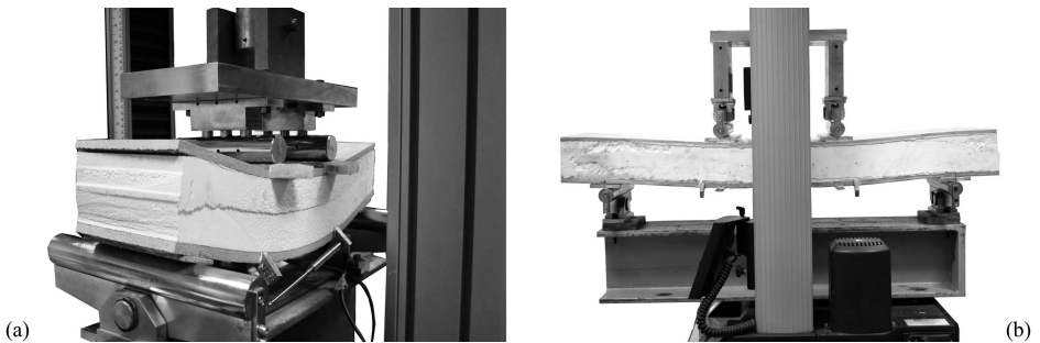
Figure 5.6: Specimens during testing: small "S" sandwich beam (a) and big "B" sandwich beam (b).
