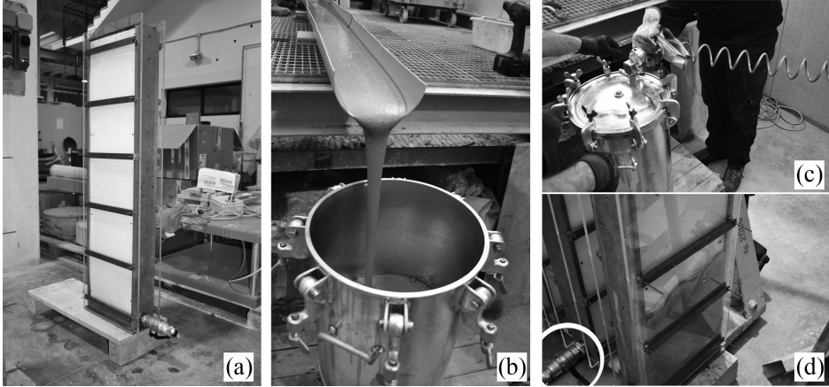
Figure 5.3: Casting of the sandwich beams: formwork with the EPS panel and the fabrics placed inside (a), tank filling (b), tank closure (c) and in-pressure injection of the mortar inside the framework (d).
