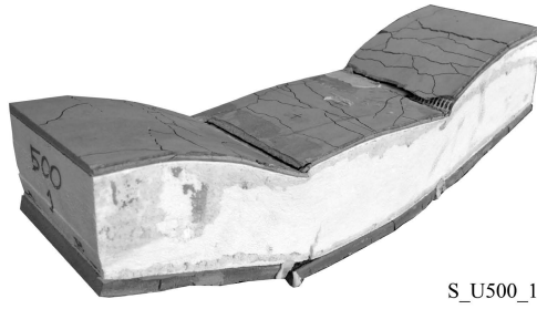
Figure 6.11: View of specimen S_U500_1 exposed to 500 cycles after test.
