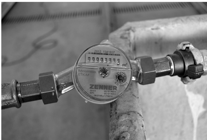
Figure 7.8: Full scale panel instrumentation: flow-meter used to measure the distributed load applied on the panel.
