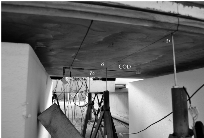
Figure 7.10: Full scale panel instrumentation: LVDTs used to measure the vertical displacement at mid-span.
