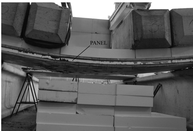
Figure 7.19: ULS full scale panel test: incipient panel failure.
