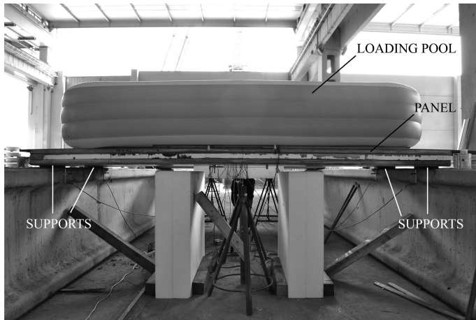
Figure 7.7: SLS full scale panel test.
