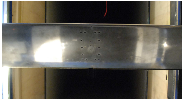
Figure 3.24: NACA 23012 blade section model inside the Politecnico di Milano wind tunnel.
