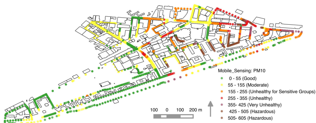
Figure 5-15 Mapping air quality using data from the mobile sensing fieldwork, example of small particles data about May 30 th . PM 10 concentration expressed in \mu\text{g}/\text{m}^3 unit, as coming from the sensor raw readings. Source: author's elaboration.
