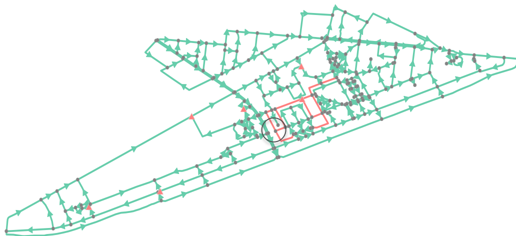
Figure 4-3 Mobile sensing path within the MIT campus. Red lines represent indoor paths while red triangles represent indoor sensing nodes. The circle corresponds to the main entrance of the campus. Source: author's elaboration.
