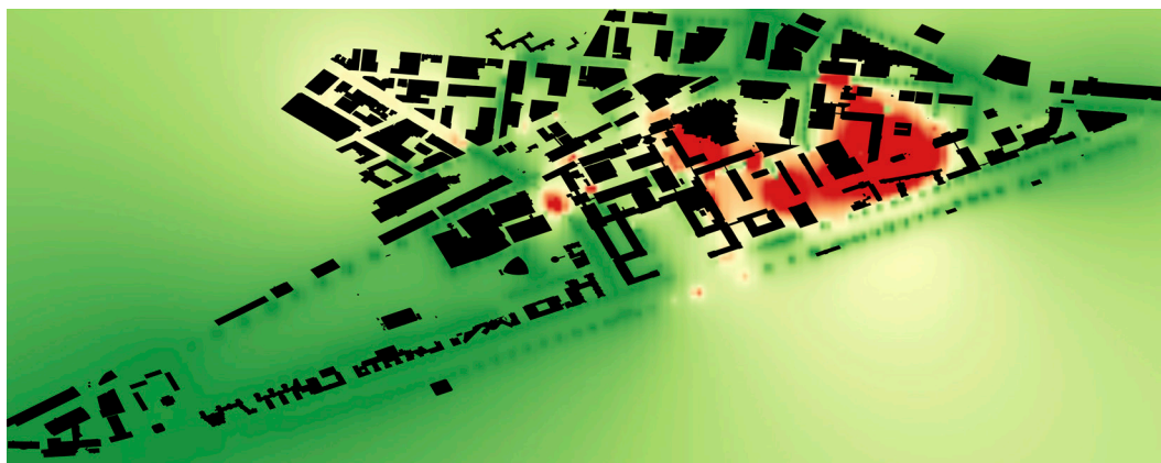
Figure 5-17 Mapping air quality using data from the mobile sensing fieldwork. Qualitative example of PM2.5 data about May 30 th . Each color represents the interpolation from all records coming from the sensor readings, according to the level of pollutant measured (red=high, green=low level). Source: author's elaboration.
