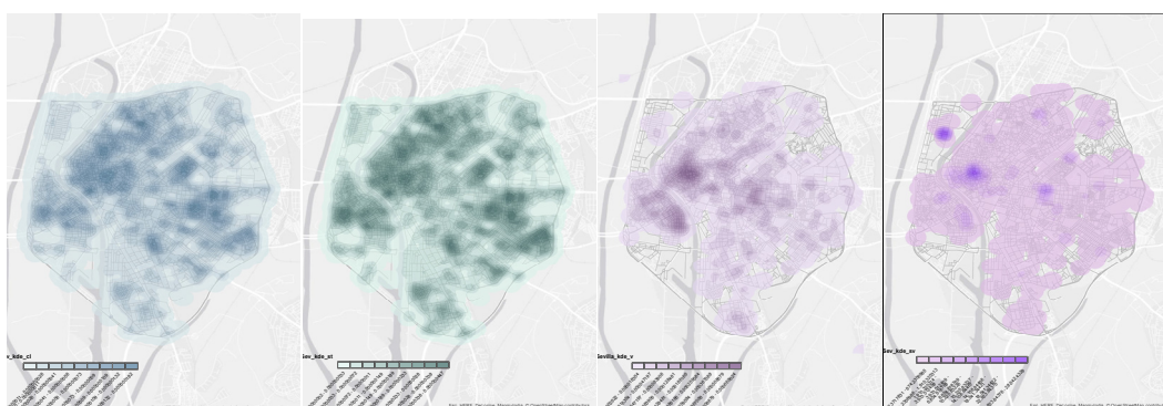
Figure 4-11 Mapping big data for exploring urban spatial pattern: Seville (Spain) urban centrality indices (closeness and betweenness, 1st and 2nd map) and correlation with activities locations (3rd map) and low correlation with sales volumes (4th map). Tools: ArcGIS and Matlab. Source: Author’s elaboration.
