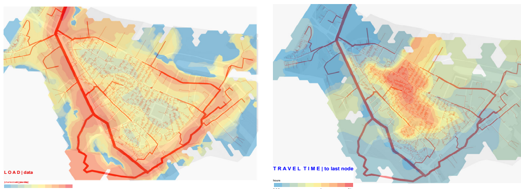
Figure 4-5 Mapping undersurface flows (load and travel time) in Charlestown, Boston, MA. Source: Author’s elaboration.
