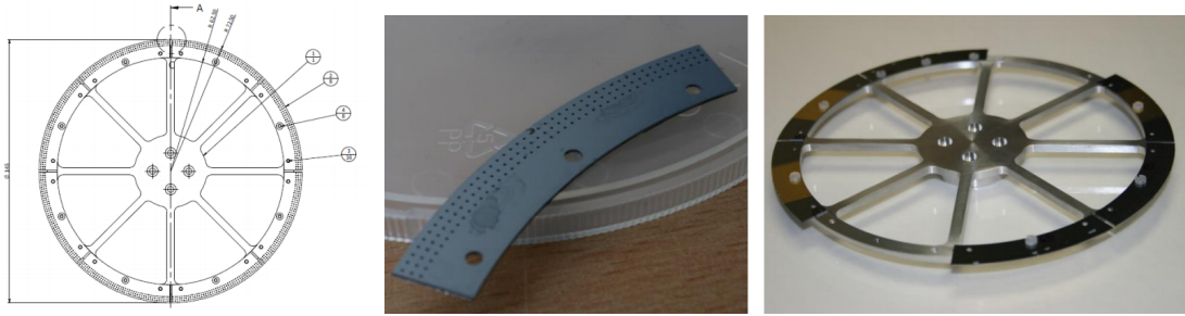
Figure 3.17: Wheel target holder geometry of RAL High Accuracy Microtargetry System: wheel schematic (left), targets arranged in rows around the wheel circumference for each sector (center), wheel main structure (right). The holder allows to position up to 1000 targets the eight segments. From [203].
