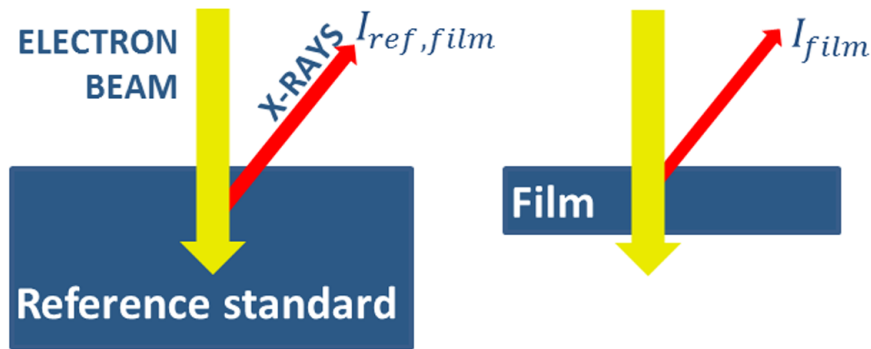
Figure 4.11: Sketch of EDS–based method for the evaluation of free–standing film areal density.
