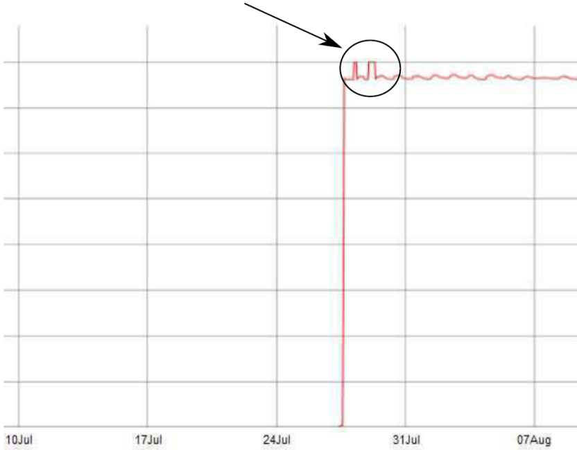
Figure 2.5: A low-probability intermittent fault at software level
